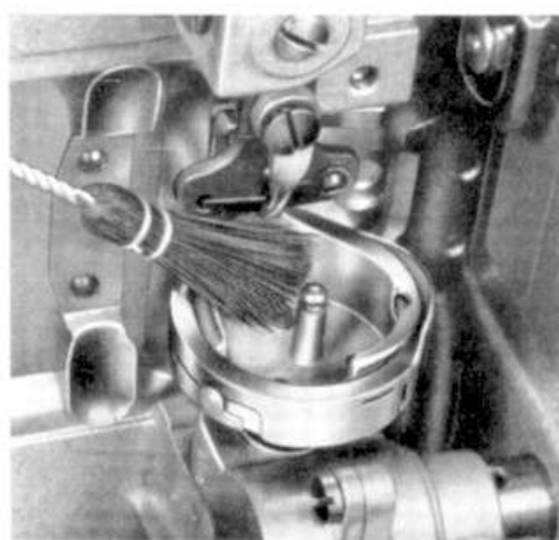
Fig. 66 Cleaning the sewing hook
