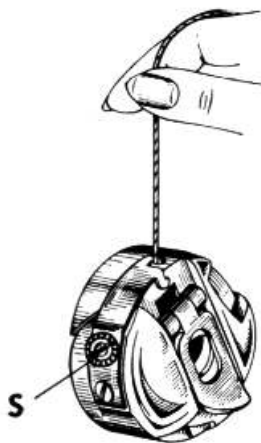
Fig. 30 Determining correct bobbin thread tension
